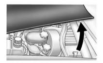
2. Go to the side of the vehicle and pull up on the rear edge of the bonnet, near the windscreen.
