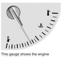
This gauge shows the engine coolant temperature.
