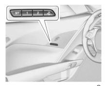
If equipped, the "1," "2," SET, and (Exit) buttons on the driver door are used to manually save and recall memory settings for the driver seat, outside mirrors, and power tilt and telescoping steering column.
