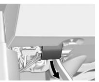
1. Pull the bonnet release lever inside the vehicle. It is below the instrument panel on the driver side.
