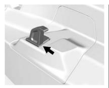
2. Insert the front of the roof panel so that the indents lie on top of the receivers.
