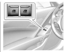
Press the switch to the first detent to lower the window. Pull to the first detent to raise the window. Release to stop at the desired position.
