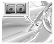
Pull up or press down on the switch to raise or lower the window. See *Power Windows on page 2-19*.
