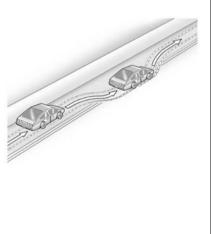
The vehicle's right wheels can drop off the edge of a road onto the shoulder while driving. Follow these tips:
