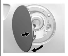
To open the fuel filler flap, push and release the rearward centre edge of the flap. The fuel door is locked when the vehicle doors are locked. Press on the RKE transmitter to unlock. With passive locking, the driver door must be opened first before the fuel door will unlock.
