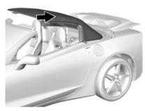
2. Lift and pivot the convertible top rearward into the fully stowed position.
