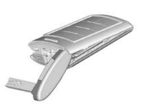
2. Use the oval base of the key blade to separate the two halves of the transmitter.
