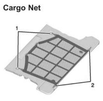
The vehicle comes with a barrier net. Unfold the net and fasten the front hooks (1) as shown to the front tie-downs in the cargo area. Pull the net over any items loaded onto the floor and fasten the rear hooks (2) to the rear tie-downs.
