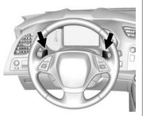
Active Rev Match (ARM) aids in smoother shifting by matching the engine speed to the next selected gear. The system is activated and deactivated by pressing either of the paddles marked REV MATCH on the steering wheel. See Active Rev Match on page 9-22.
