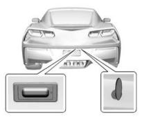
Press the hatch/boot release touch pad with the RKE transmitter within range or use the key in the key cylinder. See *Keys on page 2-1*.
