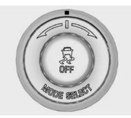
In order to select this optional handling mode, the vehicle mode must be Track. Then quickly press the TCS/StabiliTrak ab button on the centre console two times. COMPETITIVE DRIVING MODE displays in the Driver Information Centre (DIC). See *Ride Control System Messages on page 5-36*.
