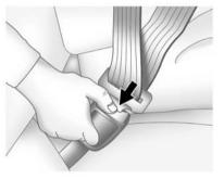
To unlatch the belt, push the button on the buckle. The belt should return to its stowed position. Before a door is closed, be sure the safety belt is out of the way. If a door is slammed against a safety belt, damage can occur to both the safety belt and the vehicle.
