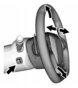
Press the control to move the tilt and telescoping steering wheel up and down or forward and rearward. Both the tilt and telescoping steering column positions can be stored with your memory settings. See *Memory Seats on page 3-4*.
