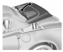
On each side of the tonneau cover, lift and pivot rearward into the fully open position.
