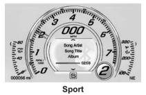
Includes a circular tachometer centred in the display. The DIC is contained within the tachometer ring. Additionally, there are two configurable pocket gauges in the lower left and right corners.
