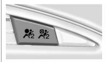
When the vehicle is started, the passenger airbag status indicator will light the symbol for on and off
