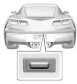
Press the release touch pad to open the boot if the RKE transmitter is within 1 m (3 ft).
