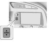
Press the button to lower the display and access the storage behind it.
