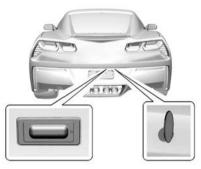
• Press the hatch/boot release touch pad with the RKE transmitter within range or use the key in the key cylinder. See Remote Keyless Entry (RKE) System on page 2-2. See Keys on page 2-1.
