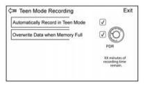
**Teen Mode Recording:** Allows the setting of recording preferences. It is recommended that a blank SD card be used. Available choices are:
