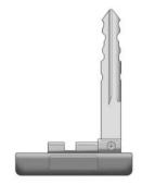
The key inside the RKE transmitter can be used to open the vehicle and tailgate/boot if power to the vehicle is lost. See *Hatch (Boot) on page 2-11*.
