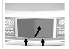
1. Press up on the two indents at the bottom and lift the aero panel off the bracket.
