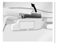
6. To unlock the front release handles, pull them outward, turning fully.
