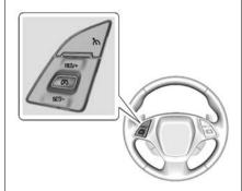
$\delta_{\Omega}$ : Press to turn cruise control on or off. A white indicator comes on in the instrument cluster when cruise is turned on. **RES/+:** If there is a set speed in memory, press briefly to resume to that speed or press and hold to accelerate. If cruise control is already active, use to increase vehicle speed.
