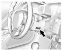
1. Place the transmitter in the steering column transmitter pocket with the chrome buttons facing up and the base toward the passenger side.
