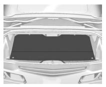
With the convertible top up, the boot partition can be unsnapped and laid flat to increase boot cargo space.
