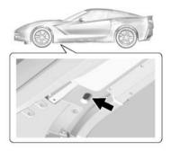
Use only a service jack with a lifting pad diameter of 64 mm (2.5 in) or smaller, and thick enough to make sure the jack does not contact the vehicle body.
