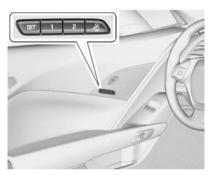
If memory equipped, the "1," "2," SET, and 🔁 (Exit) buttons on the driver door are used to manually save and recall memory settings for the driver seat, outside mirrors, and power tilt and telescoping steering column.
