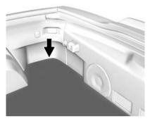
4. Open the rear hatch and lift the carpet on the passenger side of the vehicle to gain access to the battery cover.
