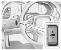
After the convertible top is completely open, a chime sounds and a DIC message displays. Release the switch.
