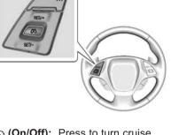
S (On/Off): Press to turn cruise control on and off. A white indicator appears in the instrument cluster when cruise is turned on.
