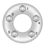
Tighten the wheel lug nuts firmly in a crisscross sequence. See *Capacities and Specifications on page 12-3.*
